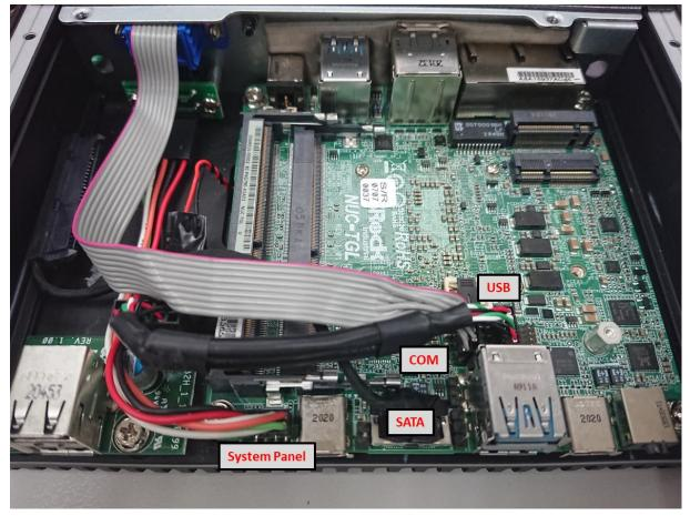
4. Remove M3x4 & M2x7.5 screws from the motherboard.
