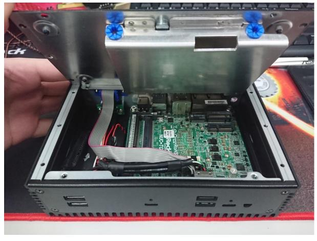
12. Tighten M3x5 screws on the bottom cover plate with torque of 3.5  $\pm$  0.5 Kgf-cm.
