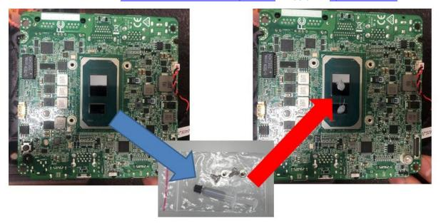
6. Paste the thermal pad on the location marked by the red rectangle below.
