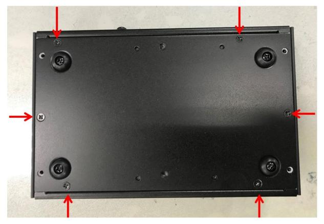
2. Remove M3x5 screws from the front panel.
